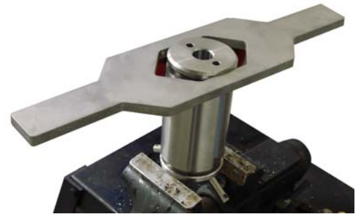
To remove bottom cap
