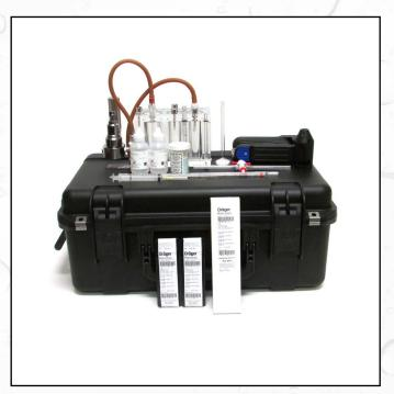
OFITE Garrett Gas Train consists of a transparent train, pressure regulator assembly,  $CO_2$  and  $N_2O$  cartridges, Dräger-Tubes<sup>TM</sup> for  $H_2S$  and carbonate detection, and a convenient carrying case. For determining active sulfides in oil-based fluids, OFITE offers a separate kit (#151-20) that analyzes whole mud samples.
