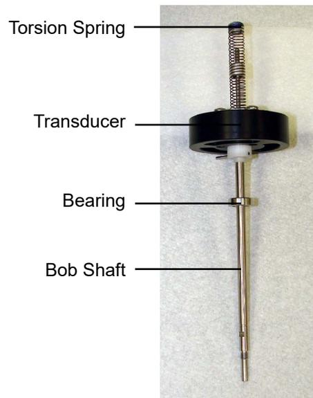
14. Insert the bob shaft back into the bearing guide. Push the transducer down onto the bearing guide so that the bearing seats in the available space.
