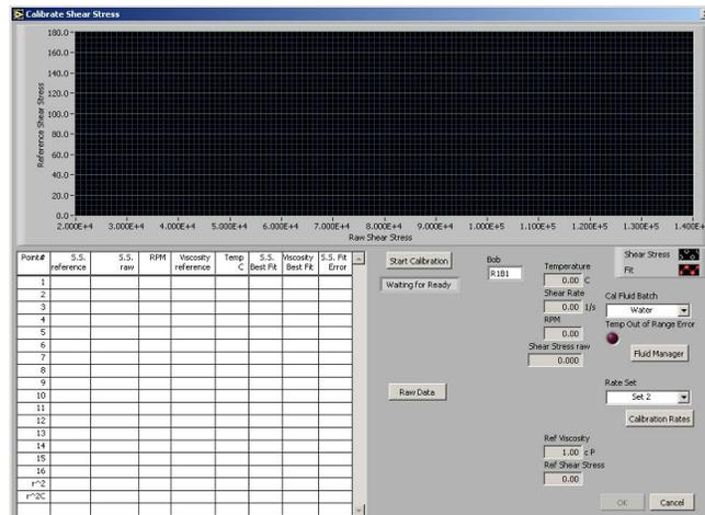
4. As the calibration proceeds, the software will begin to display the collected data in the chart. At the end of the calibration, the software will calculate the “ $r^2$ ” value, which measures the accuracy of the calibration. If this value is less than 0.9990, recalibrate the unit. If this value is still low, change the lower bearing (see page 40 for instructions) and try the calibration again. If the unit still does not calibrate, it will require servicing by an OFITE technician.
