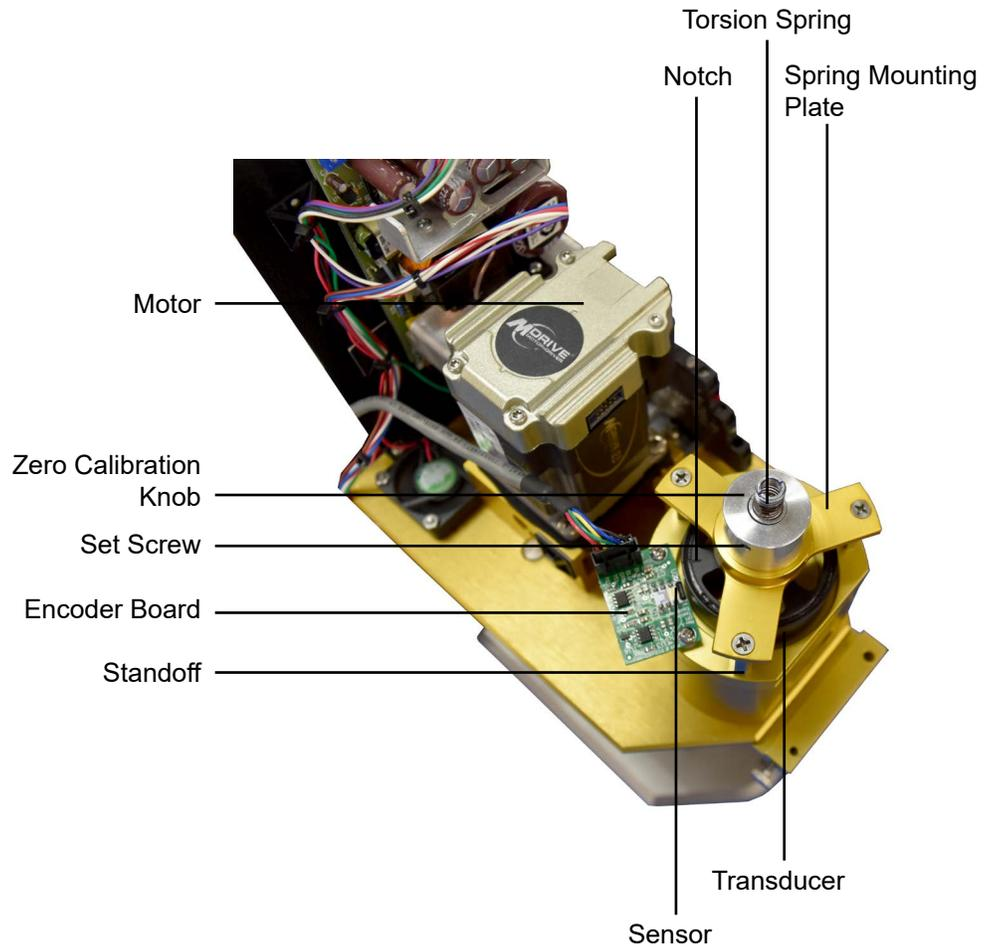
7. Remove the two screws holding the encoder board in place.
