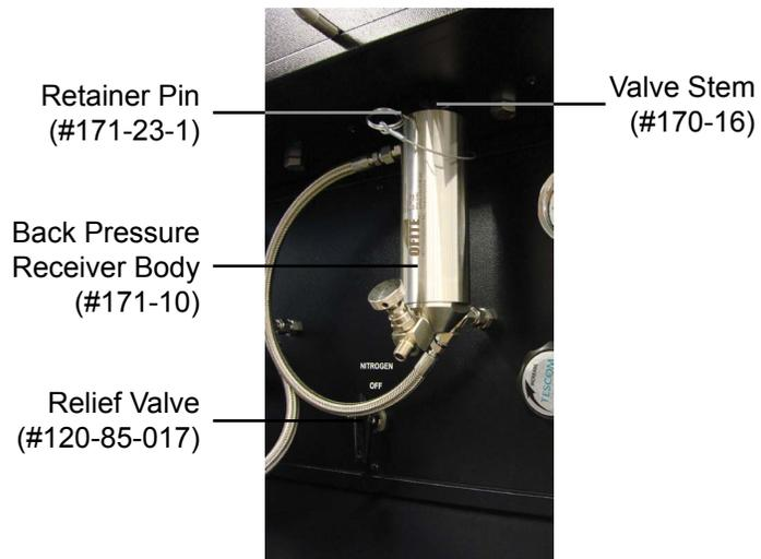
23. Connect the bottom pressure hose to the back pressure receiver (if it is not already connected). Make sure the needle valve on the back pressure receiver is closed.
