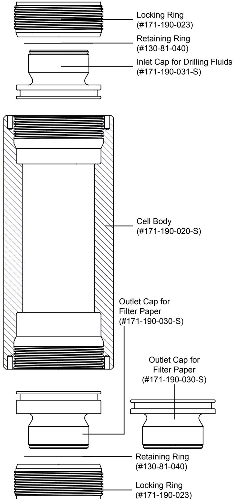
**#171-192-S - Test Cell, Stainless Steel (For Cement Testing)**
