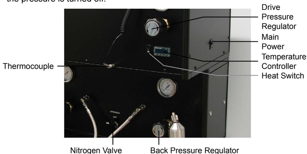
1. Before starting a test, make sure the Nitrogen valve is off (vertical). Turn off the main power switch and both heat switches. Make sure all regulators are backed off completely. Turn them completely counterclockwise.
