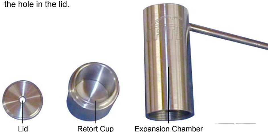
8. Lubricate the threads on the sample cup with a light coat of thread lubricant. This will prevent vapor loss through the threads and will also facilitate disassembly of the equipment at the end of the test.
