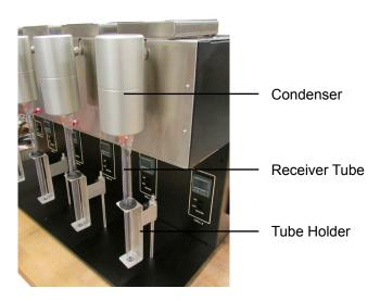
12. Set the temperature controller to 970°F (521.1°C) using the up and down arrow buttons. Turn the HEATER switch "ON". Observe the liquid exiting the condenser. Continue heating for ten minutes after condensate stops being collected.
