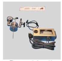
Thermocouple Assembly (#171-45-1) (Direct temperature measurement Of the fluid Inside the Cell)
