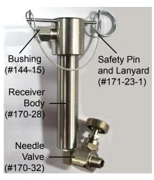
**Top Pressurization Manifold Assembly**
