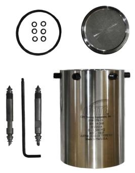
HTHP Filter Press Cell Assembly, 2000 psi, 175 mL, (#170-12-2)
