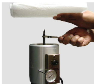
Safe Release of Pressure from a Cell
