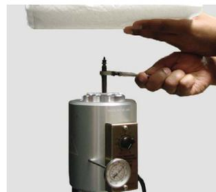
A good indication that pressure is trapped inside the cell body occurs if the cell caps are unusually difficult to loosen. To relieve any trapped pressure, an OFITE Pressure Relief Tool (#170-91) may be inserted through the inlet cell cap hole which will relieve any trapped pressure inside the cell. Ensure this function is performed on the inlet side of the cell as the filter cake may seal off the outlet end of the cell.
