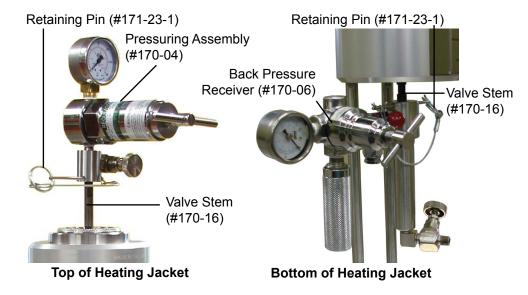
21. Keeping the valve stems closed, adjust the top and bottom regulators to the recommended back pressure for your test.
