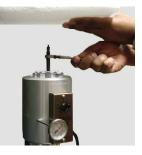
A good indication that pressure is trapped inside the cell body occurs if the cell caps are unusually difficult to loosen. To relieve any trapped pressure, an OFITE Pressure Relief Tool (#170-91) may be inserted through the inlet cell cap hole which will relieve any trapped pressure inside the cell. Ensure this function is performed on the inlet side of the cell as the filter cake may seal off the outlet end of the cell.
