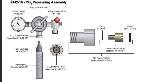
b. Regulator loses pressure or steadily increases in pressure – Replace the seat assembly and diaphragm.
