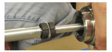
7. Carefully tap the bearing removal tool to pass the bearing spring through the bore. You should feel it clear.
