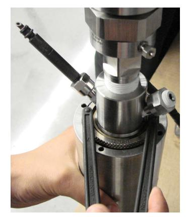
14. Screw a valve stem into the cell cap and tighten it completely.
