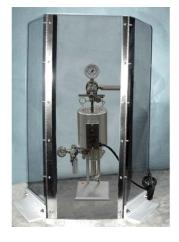
The HTHP Filter Press is a very safe instrument to operate as long as the instructions are strictly followed. It is imperative that the technician thoroughly understands the assembly and disassembly procedures and also why the order of steps is in place. Care should be taken to never use defective parts and that OFITE's temperature, pressure, and fluid volume limits are strictly adhered to at all times.
