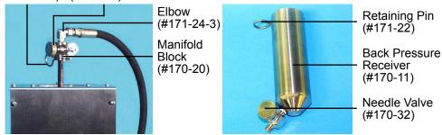
17. Keeping the valve stems closed, adjust the top and bottom regulators on the manifold to the recommended back pressure for your test.
