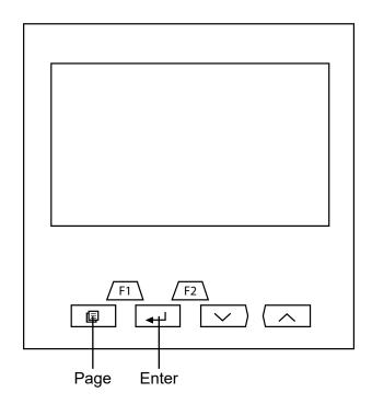
For the test described on the previous page, use the following settings Use the Enter button to decide which setting to change. Use the Arrow buttons to change the values for that setting.
