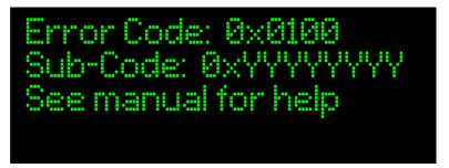
Error 0x0100 indicates a self-test failure and 0xYYYYYYY is a code specific to the type of error detected. If the self test fails, first cycle the power. If the error remains, change the batteries and/or switch to an alternate power source. If the error still remains, the meter will need to be repaired by a qualified technician.
