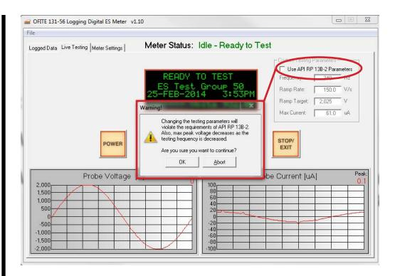
If a test must be taken outside of API parameters, uncheck the box next to "Use API RP 13B-2 Parameters". A warning will appear to inform the user that any test taken after this point will violate the requirements of API RP 13B-2.
