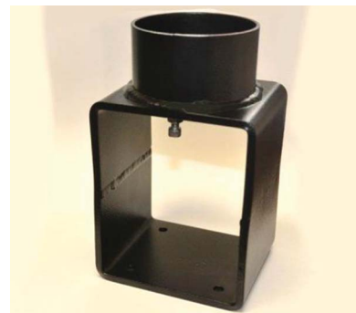
Stand for HTHP Cell Assembly (#171-190-028)
