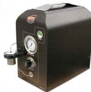
The BLP 630 Automated Gas Porosimeter is designed to rapidly and accurately measure the effective porosity of a core sample. Porosity is defined as the percentage of void space within a solid media. Effective porosity is the percentage of void -
