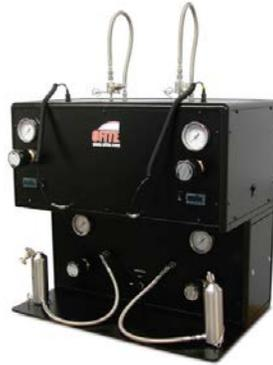
The new 2 Unit HTHP Filter Press from OFITE is ideal for high-volume laboratory testing. It accommodates two 500 mL HTHP filter press cells. Each cell has a separate electronic temperature controller and two separate pressure regulators (drive pressure and back pressure). This allows each cell to be heated and pressurized independently, while still sharing a single pressure source.
