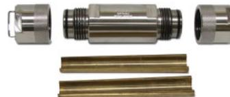
The Foam Cement Stability Tube (#122-186) is designed to cure foam cement samples at elevated temperatures while isolating the slurry from external pressure. The sealed mold prevents contamination from the pressure medium and maintains foam cement density by preventing the escape of air bubbles from the slurry.
