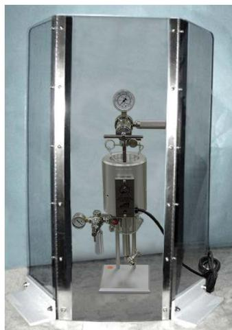
The HTHP Filter Press is a very safe instrument to operate as long as the instructions are strictly followed. It is imperative that the technician thoroughly understands the assembly and disassembly procedures and also why the order of steps is in place. Care should be taken to never use defective parts and that OFITE's temperature, pressure, and fluid volume limits are strictly adhered to at all times.
