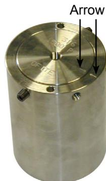
11. Use the Allen wrench to tighten the six locking set screws into the cell and secure the cell cap in place. Use hand-touch make sure that all of the set screws are completely tightened. The cell may become permanently stuck inside the heating jacket if one or more set screws are left protruding from the cell.
