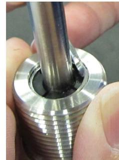
2. Unscrew the upper hex on the shaft to access bearings inside cap assembly.
