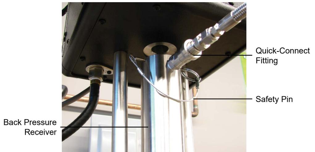
21. Connect the pressure hose from the back of the Control Box to the quick-connect fitting on the back pressure receiver.
