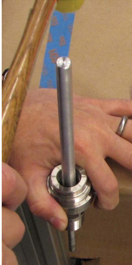
8. Insert the retaining ring. Inspect for damages to the bearing and repeat for the other bearings.
