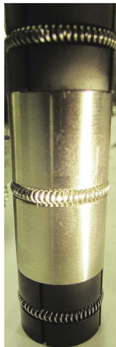
5. If necessary, reinstall the bearings while maintaining proper orientation of the springs. The direction of rotation is clockwise when viewed from the top of the drive so they must resist the rotation and be left to right when viewed from the side.
