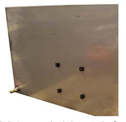
4. Tighten the four bolts to secure the drain pan to the Core Drill table.
